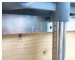
The vertical edge spacing is set exactly by way of a scale.
