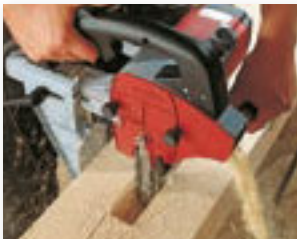
Tenon cuts of various sizes up to 100 mm (3 15/16 in.) with the LS 103 Ec.
