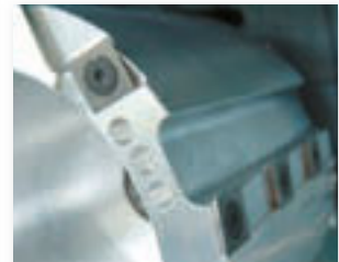
New cutter head with reversible carbide tips for extreme machining rates and optimum chip removal.
