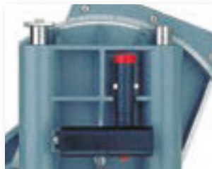
For cuts at an angle to the edge of the timber: tilt range up to 45° in both directions.
