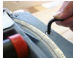
The slot mortiser can be tilted through 45° in either direction.
