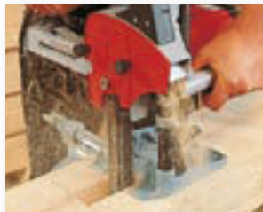
The LS 103 Ec with the guide support stand FG 150 for mortising depths of up to 150 mm (5 7/8 in.).
