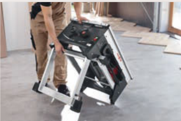
Assembling and disassembling the ERIKA are simple one-man jobs. You can unfold the built-in fold-away support within seconds and without tools. - The /Quickstand\.
