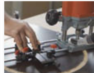
The Mafell adapter for hand router LO-FA can be used as a milling pocket stop, guide rail adapter, rip fence or compass.
