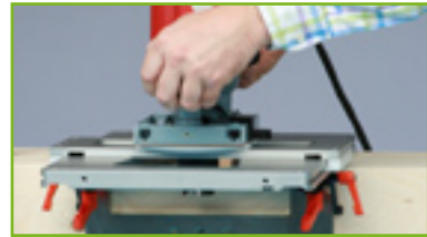
lock router cutter
