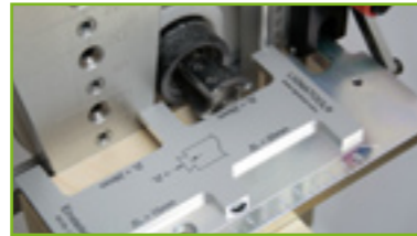
adjust milling depth
