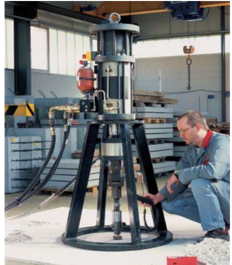
Figure 2.32: Test equipment for high load capacities
